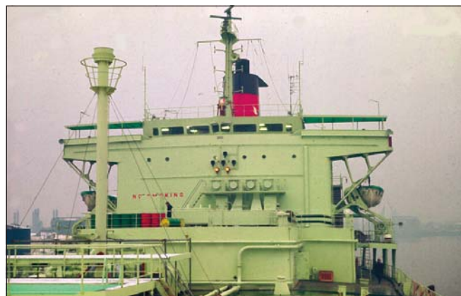
The "traffic lights" just below the wheelhouse on Faraday ; the compressor house ventilation ducting is shown below and the swimming pool in left foreground
